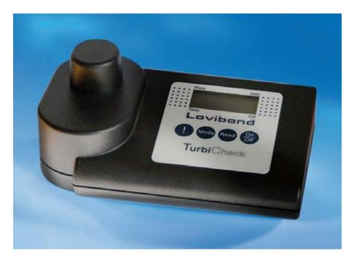
The compact Lovibond® infrared turbidity meter TurbiCheck is designed to allow fast, precise onsite testing. The unit measures the scattered light at an angle of 90°, as stipulated in EN ISO 7027.
